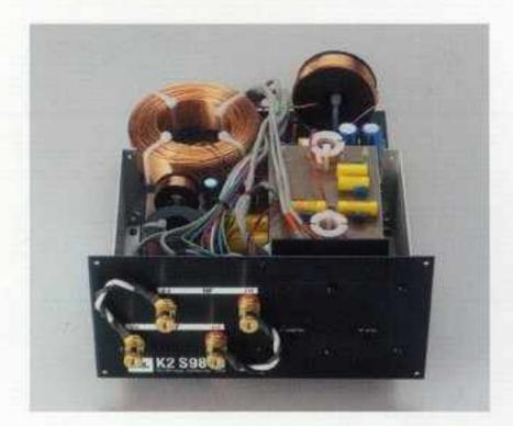
Two sets of large, gold-plated binding posts allow bi-wiring and bi-amplification. In standard connections, shorting wires with gold-plated spade plugs, located between the binding posts, prevent sonic deterioration. There's also a network bypass switch to allow active bi-amplification by separating the link between the low and high frequencies.
